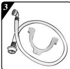
Inlet pipe + "U" elbow bracket
