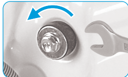
Loosen the 4 transport bolts with a spanner.
